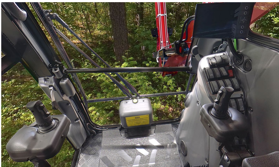
Picture 3. KESLA Vision Cabin & KESLA proC i 2.0 Electric Control System
