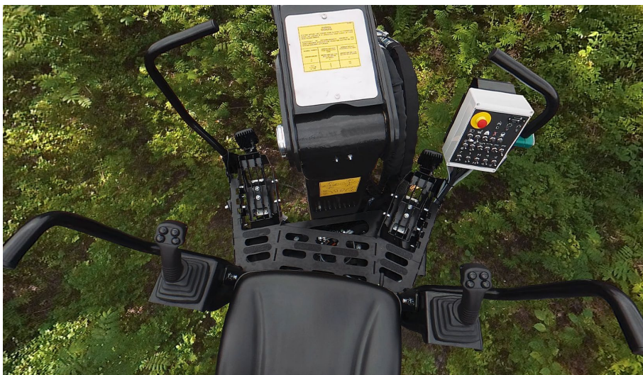
Picture 2. KESLA High Seat & KESLA proPILOT Hydraulic Control System
