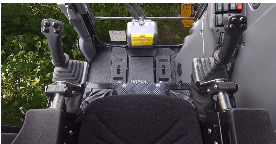
Picture 1. KESLA Vision Cabin & KESLA proPILOT 2+2 Hydraulic Control System
